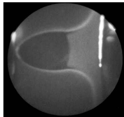
Fig. 10. Flow visualization of a supersonic free jet by LIF ( q=90 degrees, X_p=25 mm)
